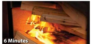
Igniter shuts down and the blower continues to push air acting as a bellow to fan the fire.
