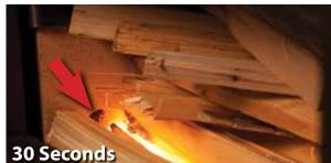
Hot surface igniter blows 1,400 degree heated air into the firebox igniting the wood.
